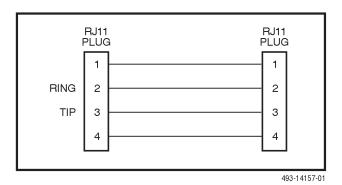
Figure D-4. Integral Modem Cable
